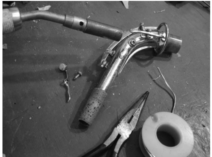
Figure 7 A chimney and sleeve for the middle Bb octave vent are soldered onto the neck.
