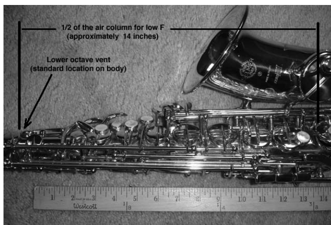
Figure 10 Measurement showing the length of the air column for low F on an alto saxophone, and the standard octave vent on the body, located approximately half-way up the air column.
